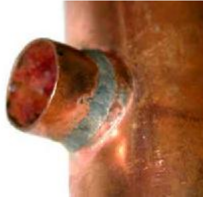
Close up of brazed header joint (CuP6 brazing rod)
